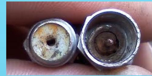
Corroded connections, connectors not tightened.
