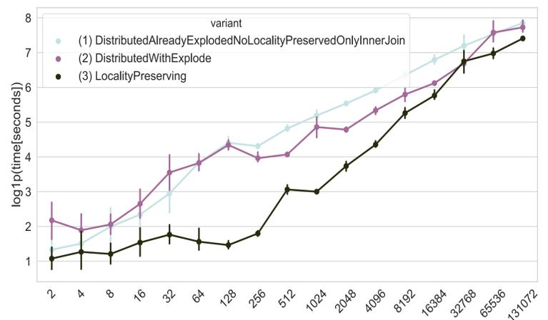
200 events per user per period for 3 periods. Load of users (x axis), processing time shown in logarithmic scale (y axis) for the 3 different implementations of a spatial join. Each one was run 5 times. The graph shows the mean and 95% confidence intervals as error bars.
