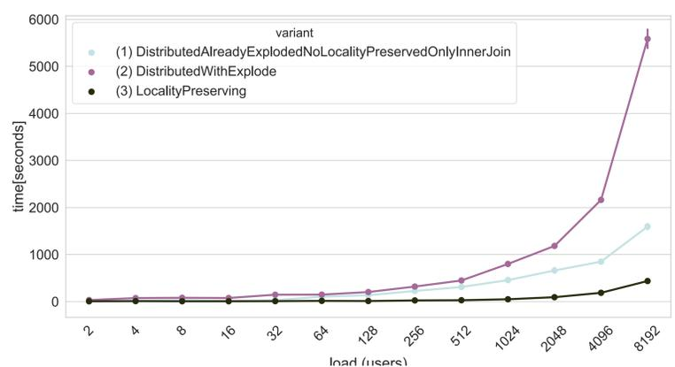
Increased number of events per user to 2000 events per period for 3 periods. Load of users (x axis), processing time shown in seconds (y axis), 5 runs each.
